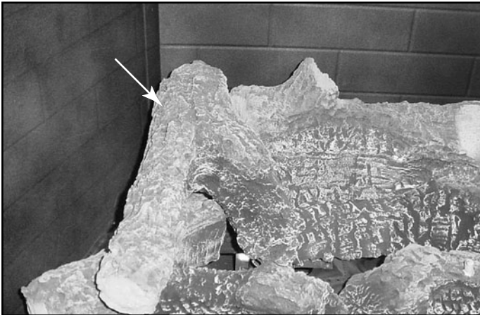
Figure 14.6 Placing Left Top Log
