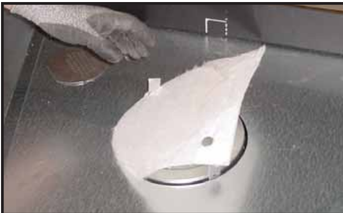
Figure 9.3 Remove the white gasket material covering the seal cap.
