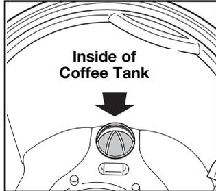
1. Lift up on screen to remove it from coffee tank. Rinse screen under stream of water to flush screen clean.
