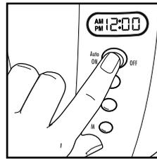
6. Wait 20 minutes to allow the descaler to clean. Then turn ON again. When the brew cycle is finished, turn OFF. Wait for BrewStation and water in coffee tank to cool, then empty coffee tank and rinse.
