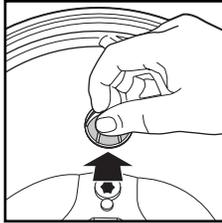
2. The screen snaps back into position over the seal in coffee tank.
