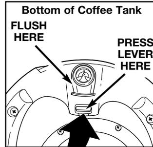
Over the sink, turn the coffee tank upside-down then press lever and flush with water for 30 seconds to remove coffee grounds.
