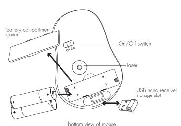
Remove the battery compartment cover, install the 2 supplied AAA batteries, then replace the cover.
