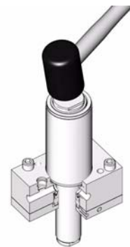
Seat Cylinder in Bore TI9108a
