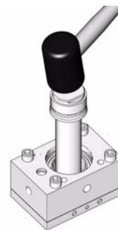
FIG. 13: Insert Rod through Throat Seal
