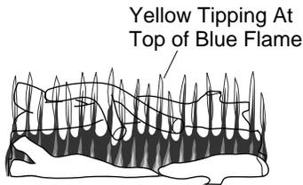
**Figure 29 - Incorrect Front Burner Flame Pattern**
