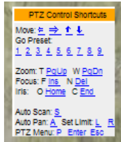
Diagram 2.13 PTZ control keys and functions
