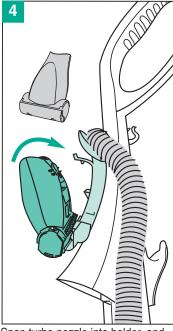
Snap turbo nozzle into holder, and loop hose on front of handle.
