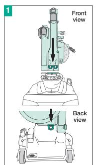
Place vacuum back on base and push down until it snaps into place.
