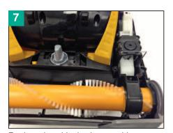
Replace the white latch assembly back into position.
