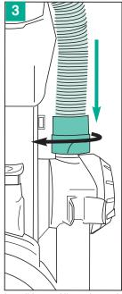
Install hose: Align tabs and push down; twist clockwise to lock.
