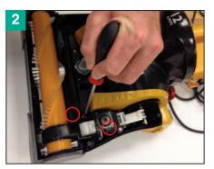
Use a Phillips screwdriver to remove 2 screws.
