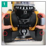
Remove 4 screws from brush roll cover. Lift off cover using rear tabs.
