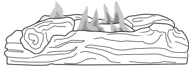
Figure 48 - Correct Burner Flame Pattern
