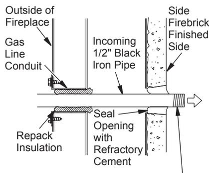
Provide Enough Threaded End for Fitting Connection
