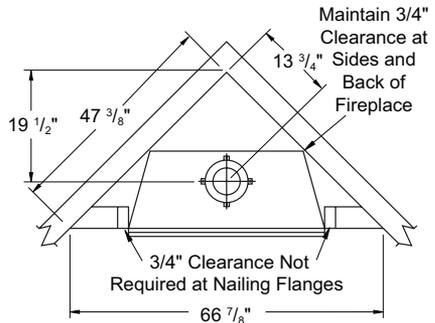
Figure 2 - Corner Installation
