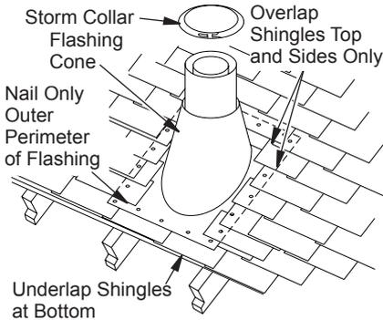
Figure 15 - Flashing Installation
