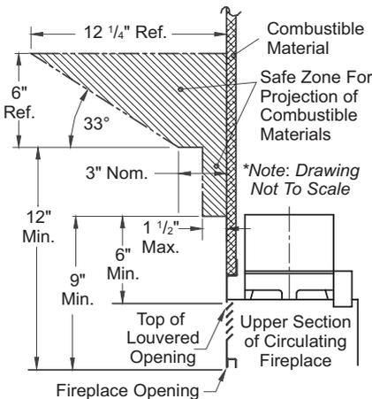
Figure 4 - Mantel Clearances to Combustible Material
