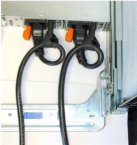
Figure 3: Routing Power Cables Through the Strain Reliefs
