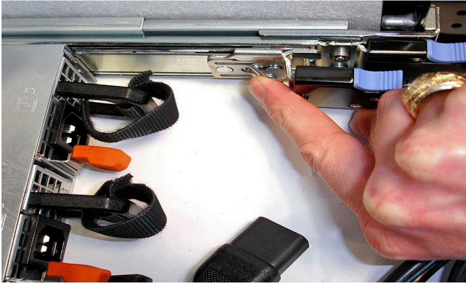
Figure 11: Replacing the Outer Power Supply
