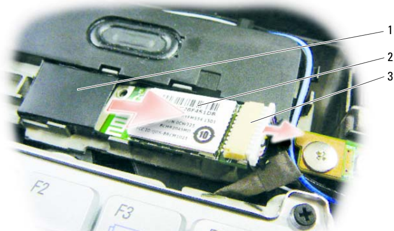
1 box 2 card 3 cable connector
