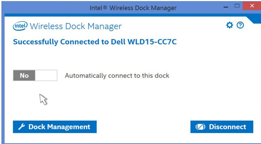
Figure 14. Choose No to not connect automatically
