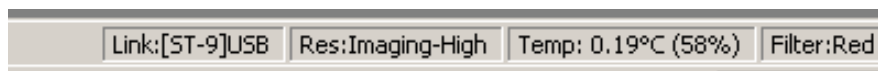
Figure 3. CCDOps status bar (from lower left corner of CCDOps desktop). This example shows (from left to right): an established link, normal unbinned (high resolution) imaging, and the temperature setpoint set to 0.19 degrees C. The cooling capacity gauge reads 58% capacity, and there is a red filter in the beam.
