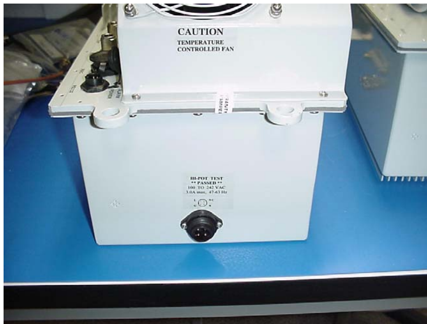
Figure 4 - AC Power Connection
