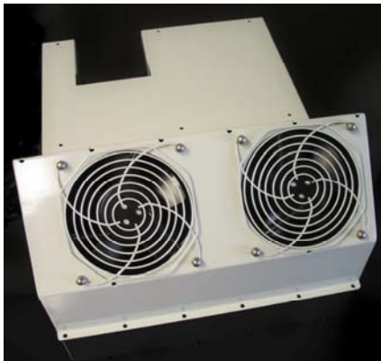
Figure 7 - Fan shroud removed from SSPA
