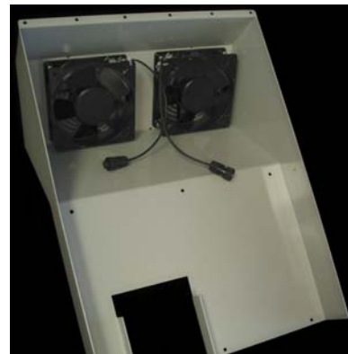
Figure 8 - Underside of fan shroud
