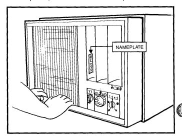
While one person holds back of casing, second person slides chassis out from casing. **NOTE:** Coil fins on chassis are sharp and chassis is heavy.
