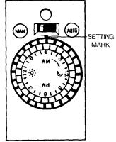
Timer pins are positioned inwards (toward center of dial) from factory to allow continuous operation.
