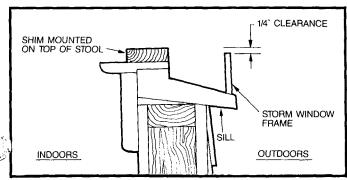
If storm windows present interference, fasten a 2" wide wood strip to window's sill. Thickness of wood strip should equal height of storm window's ledge. By inserting wood strip, you will create a level surface for unit installation.
