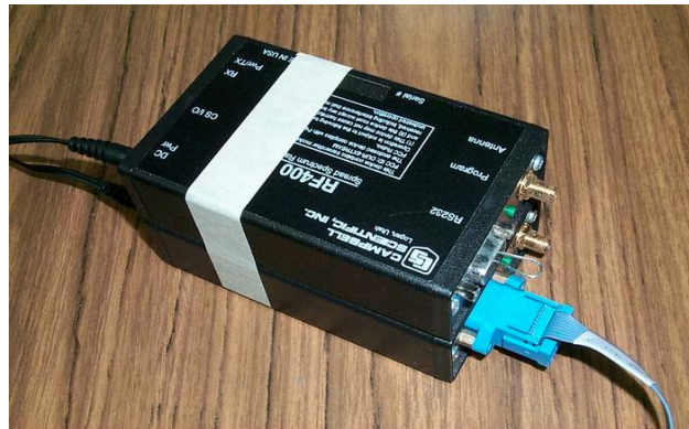
FIGURE K-1. Loop-back Test without Antennas
