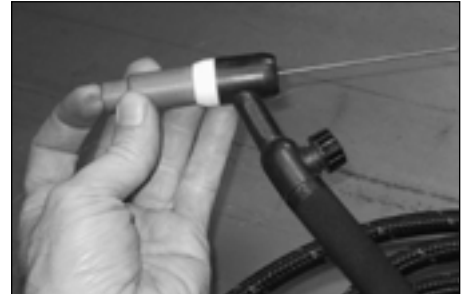
Figure 4 - Tungsten should stick out 3/16"
