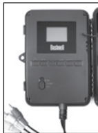
Cable from "A/V Out"
