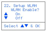
Press ( ▲ ) or | ▼ | to choose on (or off), then press **OK**. The wired network interface will become inactive with this setting.
