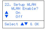
Press ( ▲ ) or ( ▼ ) to choose on (or off), then press OK. The wired network interface will become inactive with this setting.
