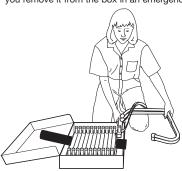
4. Place the folded sill hooks on top of the rungs, between the standoffs as shown in the diagram.
