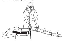
Use the plastic strap (attached to the last rung) to wrap and secure the rungs. This will minimize the chance of the ladder becoming tangled when you remove it from the box in an emergency.
