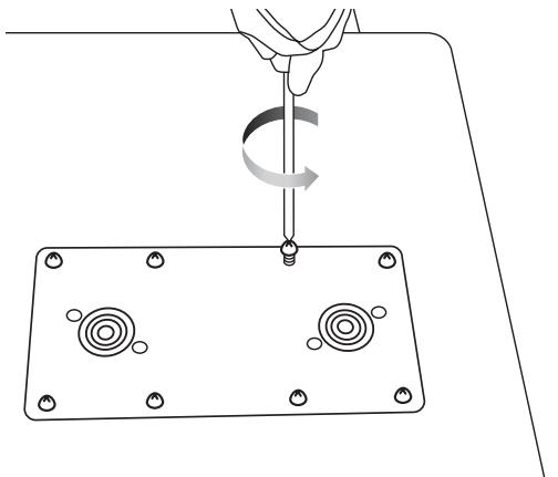
1. Remove the rear connector plate.
