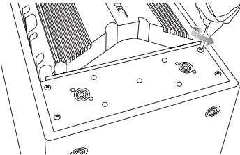
1. Remove the rear connector plate.
