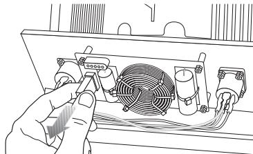
2. Remove connector from the passive position.
