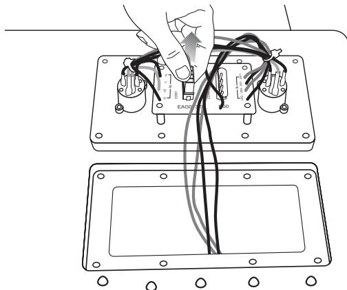
2. Remove the connector from the passive position.
