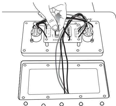
1. Remove the rear connector plate.
