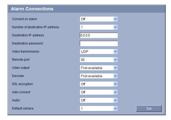
You can select how the module responds to an alarm. In the event of an alarm, the unit can automatically connect to a pre-defined IP address. You can enter up to ten IP addresses which the module will select in order, until a connection is made.
