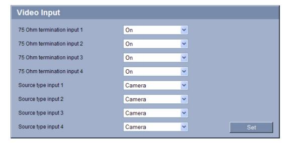
You can activate the 75 Ohm terminating resistor for each video input on the module. The terminating resistance must be deactivated for the video signal to be looped through. Every video input is closed at the time of delivery.
