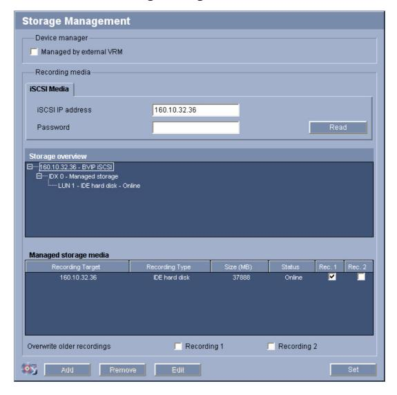
You can record the images from the camera connected to the module on an appropriately configured iSCSI system.
