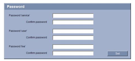
A module is generally protected by a password to prevent unauthorized access to the unit. You can use different authorization levels to limit access.
