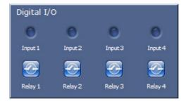
The alarm icons **Input 1** to **Input 4** are for information purposes and indicate the status of an alarm input: When an alarm is triggered, the corresponding icon lights up blue. The unit's configuration determines whether the alarm is displayed, as well as additional details (see *Section 5.15 Advanced Mode: LIVEPAGE Functions, page 40*).
