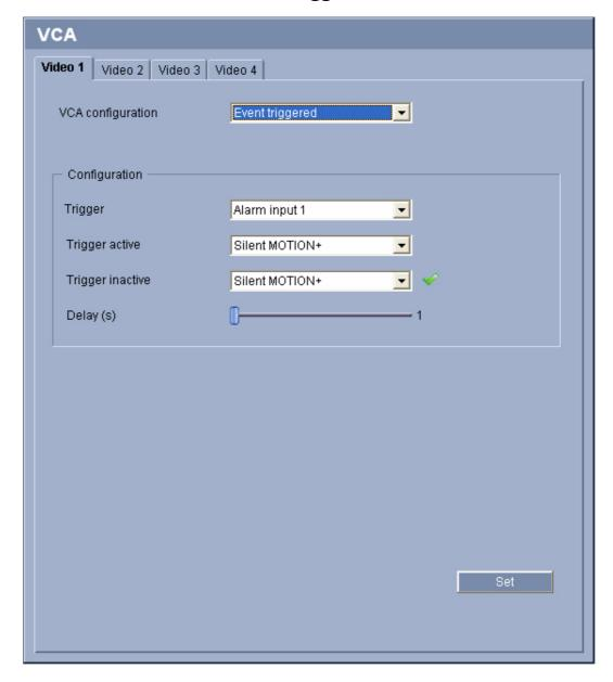
This configuration allows you stipulate that the video content analysis is only to be activated when triggered by an event. As long as no trigger is activated, the **Silent MOTION+** configuration in which metadata is created is active; this metadata facilitates searches of recordings, but does not trigger an alarm.
