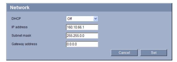
The settings in this screen are used to integrate the module into an existing network. Some changes only take effect after the module is rebooted. In this case, the **Set** button changes to **Set and Reboot**.
