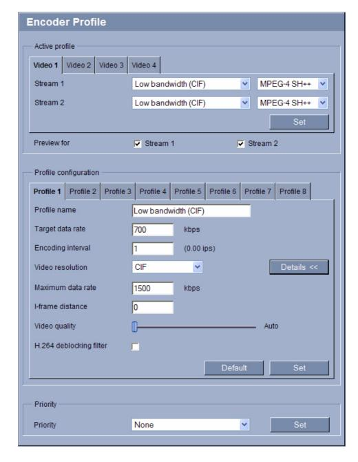
For the video signal encoding, you can select two profiles and a code algorithm for each video input, and you can change the presets for the profiles.
