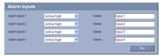
You can configure the alarm inputs for the module.
