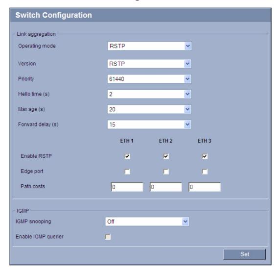
The parameters on this page can be used to configure the switch integrated into VIP X1600 XF and adapt it to the network. If several Ethernet interfaces of the VIP X1600 XF are connected with the network, you can use different protocols to optimize data transfer. Detailed knowledge of the network in which the VIP X1600 XF is located is essential in order to configure the parameters on this page.
