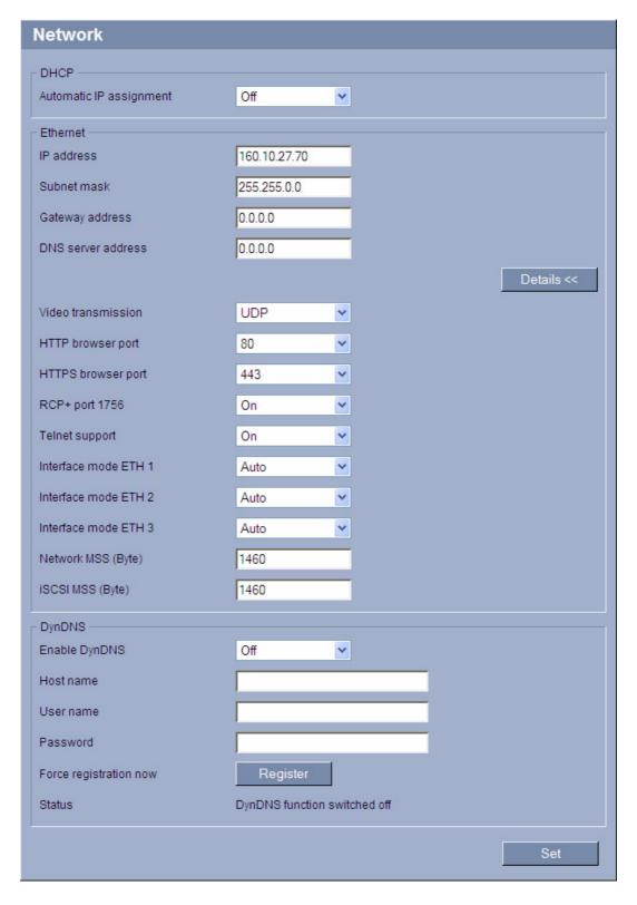
The settings in this screen are used to integrate the module into an existing network. Some changes only take effect after the unit is rebooted. In this case, the **Set** button changes to **Set and Reboot**.
