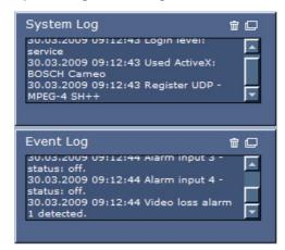
The **System Log** field contains information about the operating status of the module and the connection. You can save these messages automatically in a file (see *Section 5.15 Advanced Mode: LIVEPAGE Functions, page 40*).
