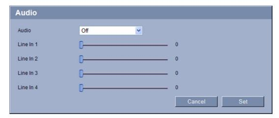
You can set the gain of the audio signals to suit your specific requirements. The current video image is shown in the small window next to the slide controls to help you check the audio source and improve assignments. Your changes are effective immediately.
