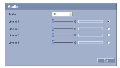
You can set the gain of the audio signals to suit your specific requirements. The current video image is shown in the small window next to the slide controls to help you check the audio source and improve assignments. Your changes are effective immediately.
