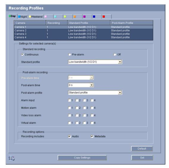
You can define up to ten different recording profiles. You will then use these recording profiles in the recording scheduler, where they are linked with the individual days and times (see Section 5.24 Advanced Mode: Recording Scheduler, page 53).
