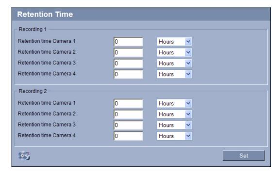
You can specify the retention times for recordings. If the available memory capacity of a medium has been used, older recordings are only overwritten if the retention time entered here has expired.
