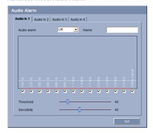
The module can create alarms on the basis of audio signals. You can configure signal strengths and frequency ranges in such a way that false alarms, for example due to machine noise or background noise, are avoided. Configure the required settings for each audio input.
