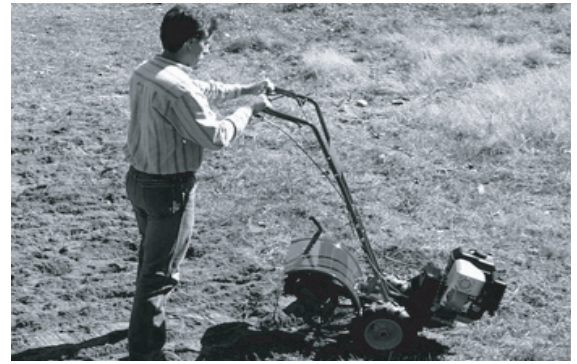
Figure 4-4: To begin turn, lift handlebars until tines are out of ground and unit is balanced.
