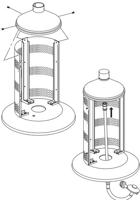
Line up 3 holes in Cap Assembly with holes in top of Shroud and legs.
