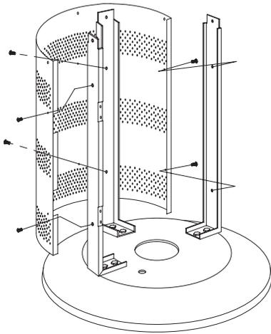
Line up slots in Cylinder Shroud flange with notches in left leg as shown.
