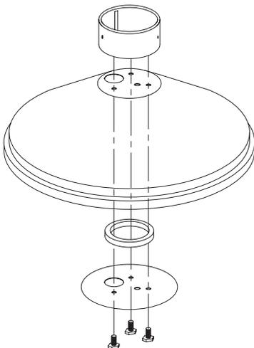
Place Spacer Ring on Support Plate so that all holes in plate fit inside ring.
