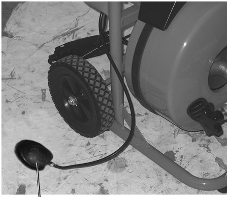
Pneumatic Foot Pedal (14A): Press On, release Off
