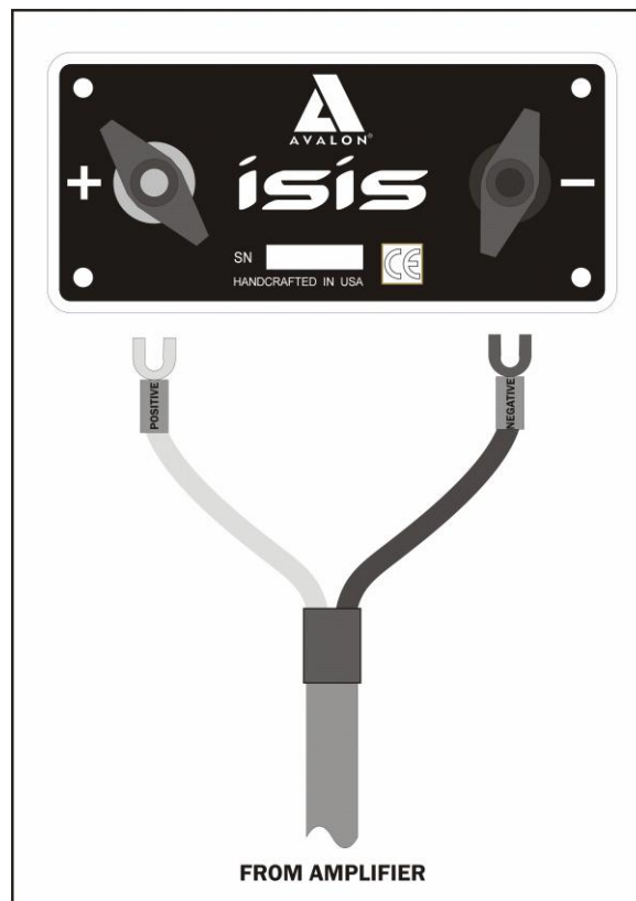
Figure 3.1 - Back view of the speakers showing the connections from the amplifier to the loudspeaker. Check to insure the correct polarity (positive lead connected to the (+) terminal and negative lead connected to the (-) terminal).
