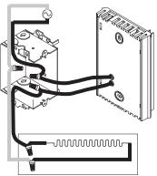
Install the base onto an electrical box.
