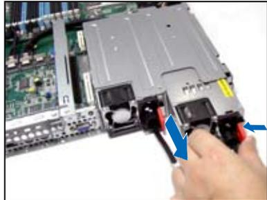
4. Firmly push the new power supply module into the chassis until the latch locks to the server chassis.
