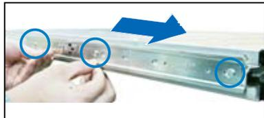
2. Secure the front end of the server rail to the side of the chassis with one screw.
