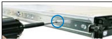
3. Attach the rear end of the server rail to the side of the chassis, matching each of the two hooks to the holes on the rail. Then slide the rail toward the front panel until it locks in place.
