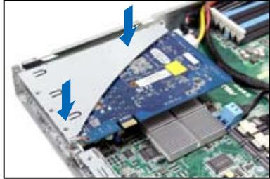
To install a PCI Express x8 or x16 card in PCIE2 slot:
