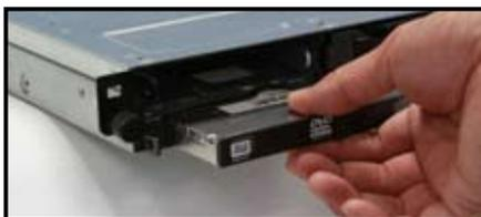
5. Carefully insert the replacement optical disk drive module into the drive bay until it is securely seated in place.
