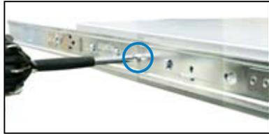
5. Repeat steps 1 to 4 to attach the second server rail to the other side of the chassis.
