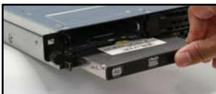
6. Carefully insert the drive tray and push it all the way to the depth of the bay until just a small fraction of the tray edge protrudes.
