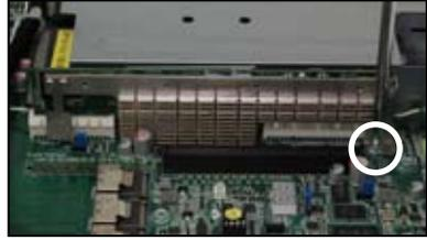
6. Disconnect the data cable from ISATA1 and connect it to the PSAS1 connector.
