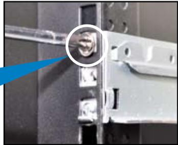
7. When mounting the server to the rack, ensure to include the side knots on the two sides of the server in the rack rail holders, as shown in the right figure.
