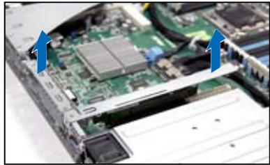
2. Place the riser card bracket on a flat and stable surface, then remove the screw from the slot bay.
