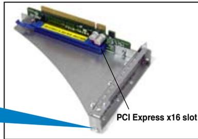
3. Install a PCI Express x8 or x16 card to the bracket as shown, then secure the card with a screw.
