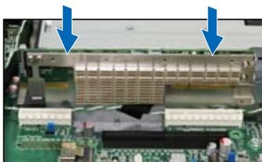
5. Secure the RAID card with the screw that you removed earlier.
