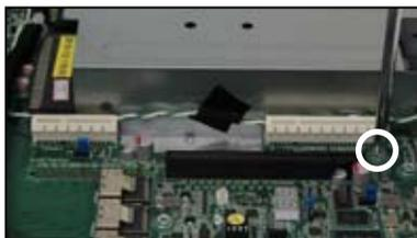
4. Align the golden fingers of the RAID card with the PIKE1/PIKE2 RAID card slots then carefully insert the RAID card into the slots.
