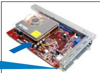
To reinstall the riser card bracket in PCIE2 slot:
