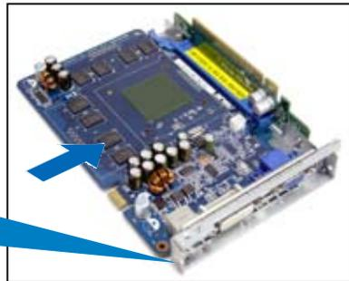
To reinstall the riser card bracket in PCIE1 slot:
