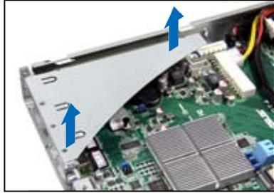
2. Place the riser card bracket on a flat and stable surface, then remove the screw from the slot bay.
