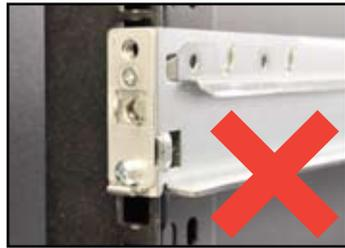
**DO NOT** install the rail to the outer side of the server rack.
