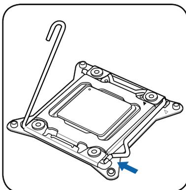
10. Push down the left load lever (L), and then insert the lever under the retention tab (M).
