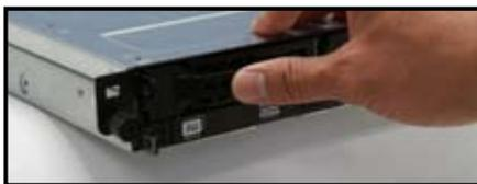
7. Push the tray lever until it clicks, and secures the drive tray in place. The drive tray is correctly placed when its front edge aligns with the bay edge.
