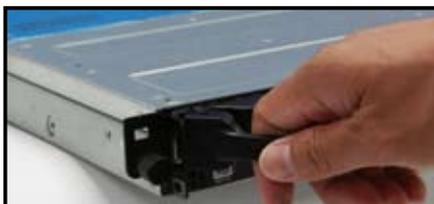
3. Firmly hold the tray lever and pull the drive tray out of the bay.
