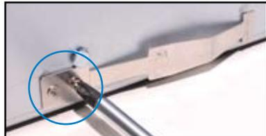
2. Select a 1U space on the rack where you want to install the rack rail. A 1U space consists of three square mounting holes with two thin lips on the top and the bottom, as shown in the right figure.
