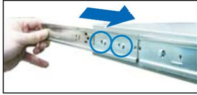
4. Secure the rear end of the server rail to the side of the chassis with one screw.
