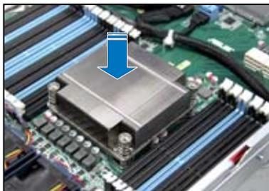
2. Twist each of the four screws with a Philips (cross) screwdriver just enough to attach the heatsink to the motherboard. When the four screws are attached, tighten them one by one to completely secure the heatsink.
