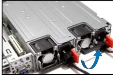
2. Hold the power supply module lever and press the PSU latch.
