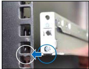
5. Secure the front and rear ends of the rail with two rack screws and washers.
