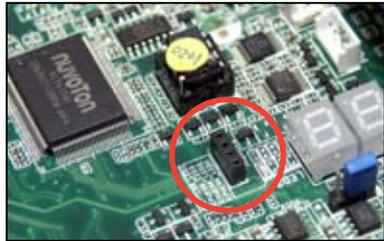
2. Connect the ASRK module to the connector.
