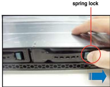
2. Firmly hold the tray lever and pull the drive tray out of the bay.
