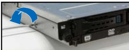
2. Remove the SATAII/SAS drive tray by pushing the spring lock to the right, then pulling the tray lever outward. The drive tray ejects slightly after you pull out the lever.
