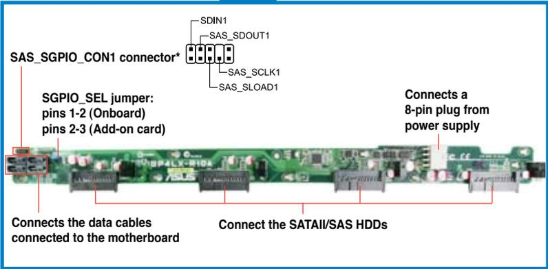
\* For PIKE RAID solution, ensure to connect SAS\_SGPIO\_CON1 to the SGPIO1 connector on the motherboard.
