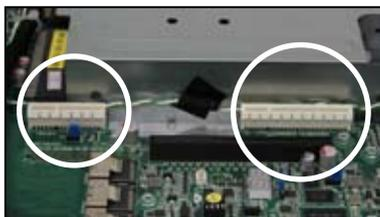
3. Remove the screw beside the PIKE1 slot on the motherboard. Keep it for reassembly.
