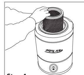
Step 4 First remove HEPA filter by placing your hand on the inner side of the filter. Then pull up gently until totally out.
