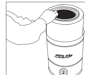
Step 5 Now remove Carbon filter by placing hands on the inner side of the filter. Then pull up gently until totally out.
