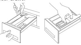
the drawer from the machine, press the button in the rear left-hand corner.
