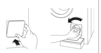
Place a container under the filter and unscrew it; some water will come out of the filter.
