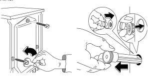
Plug the open holes with the plugs which you will find at the back of the appliance.
