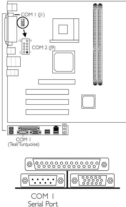
The built-in serial ports are RS-232C asynchronous communication ports with 16C550A-compatible UARTs that can be used with modems, serial printers, remote display terminals, and other serial devices. You can set the serial ports' I/O address in the Integrated Peripherals submenu ("Super IO Device" field) of the BIOS.
