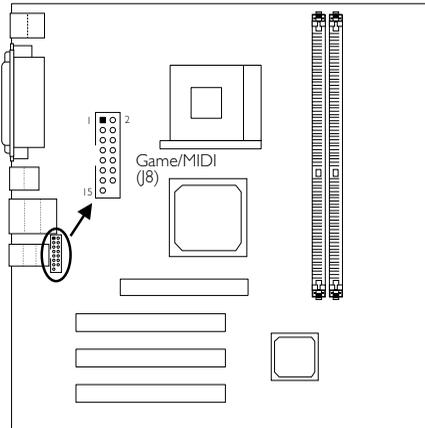
The system board is equipped with a 15-pin connector at location J8 for connecting an external game/MIDI port. One card-edge bracket, mounted with a serial port cable and a game/MIDI port cable, is provided with the system board. Install the card-edge bracket to the system chassis then connect the game/MIDI port cable to connector J8. Make sure the colored stripe on the ribbon cable is aligned with pin 1 of connector J8.
