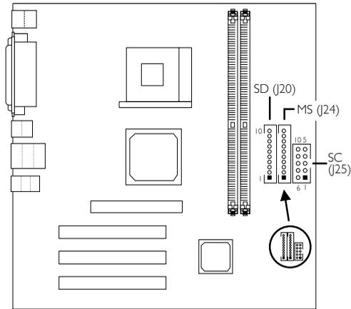
The PM1 I-UL/RAMA mainboard is equipped with a security interface - Smart Card (SC) interface and two compact storage interfaces - Memory Stick (MS) interface and Secure Digital Memory Card (SD) interface. An optional device will be provided allowing you to insert these cards.
