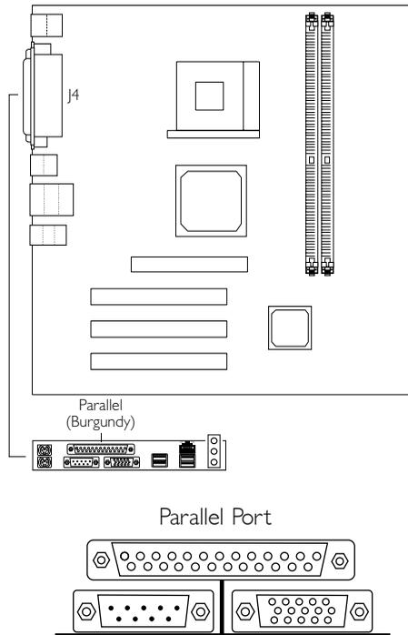
The mainboard has a standard parallel port (J4 - Burgundy) located at the ATX double deck ports of the board for interfacing your PC to a parallel printer. It supports SPP, ECP and EPP modes. You can select the port's mode in the Integrated Peripherals submenu ("Super IO Device" field) of the BIOS.
