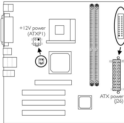
We recommend that you use a power supply that complies with the ATX12V Power Supply Design Guide Version 1.1. Connect the ATX12V power supply's 20-pin ATX main power connector and 4-pin +12V power connector to J26 and ATXP1 respectively.
