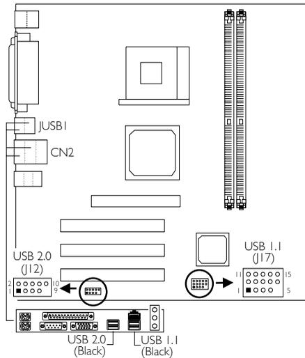
The PM11-UL/RAMA mainboard is equipped with two onboard USB 2.0 ports (JUSB1 - Black) and two onboard USB 1.1 ports (CN2 - Black) located at the ATX double deck ports of the board.
