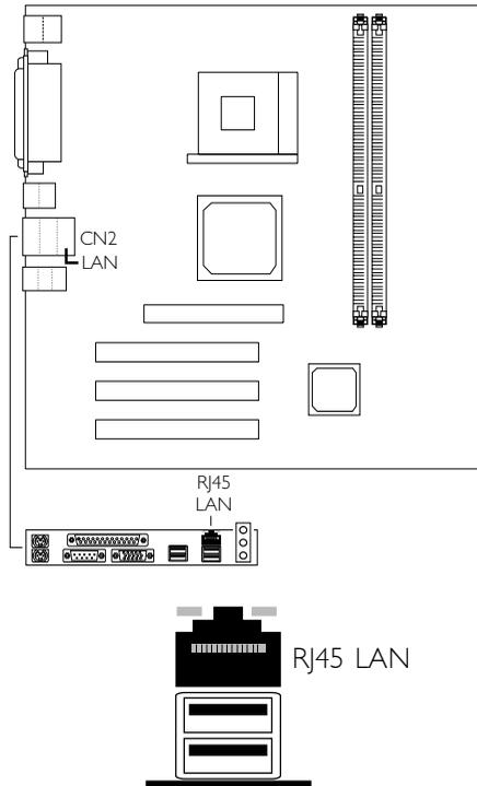
The PM11-EL/RAMA and PM11-UL/RAMA mainboards are each equipped with an onboard RJ45 fast-ethernet LAN port at location CN2 of the ATX double deck ports. It allows the mainboard to connect to a local area network by means of a network hub. You may enable or disable the onboard LAN in the Integrated Peripherals submenu ("VIA OnChip PCI Device" field) of the BIOS.
