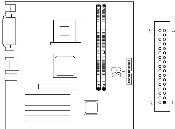
The mainboard is equipped with a shrouded floppy disk drive connector that supports two standard floppy disk drives. To prevent improper floppy cable installation, the shrouded floppy disk header has a keying mechanism. The 34-pin connector on the floppy cable can be placed into the header only if pin 1 of the connector is aligned with pin 1 of the header. You can enable or disable this function in the Integrated Peripherals submenu ("Super IO Device" field) of the BIOS.
