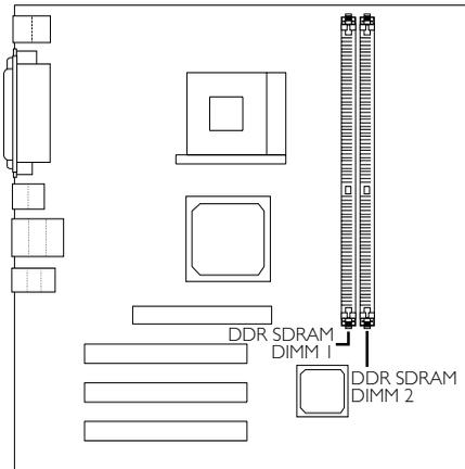
The mainboard is equipped with two 184-pin DDR SDRAM DIMM (Dual In-line Memory Module) sockets that support 2.5V DDR SDRAM DIMM. Double Data Rate SDRAM (DDR SDRAM) is a type of SDRAM that doubles the data rate through reading and writing at both the rising and falling edge of each clock. This effectively doubles the speed of operation therefore doubling the speed of data transfer.
