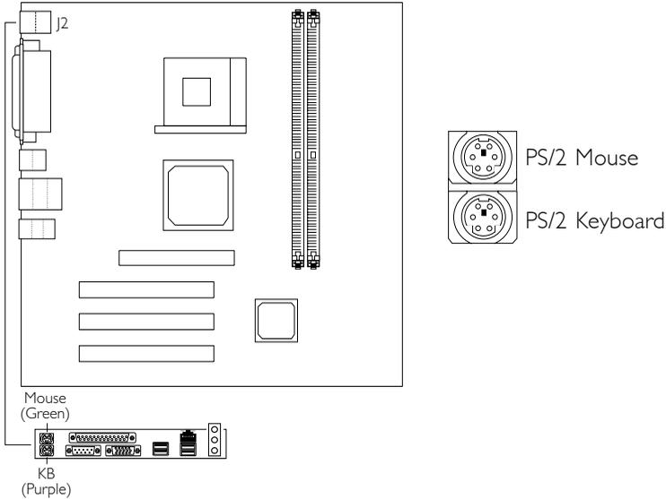
The mainboard is equipped with an onboard PS/2 mouse (Green) and PS/2 keyboard (Purple) ports - both at location J2 of the ATX double deck ports of the mainboard. The PS/2 mouse port uses IRQ12. If a mouse is not connected to this port, the system will reserve IRQ12 for other expansion cards.
