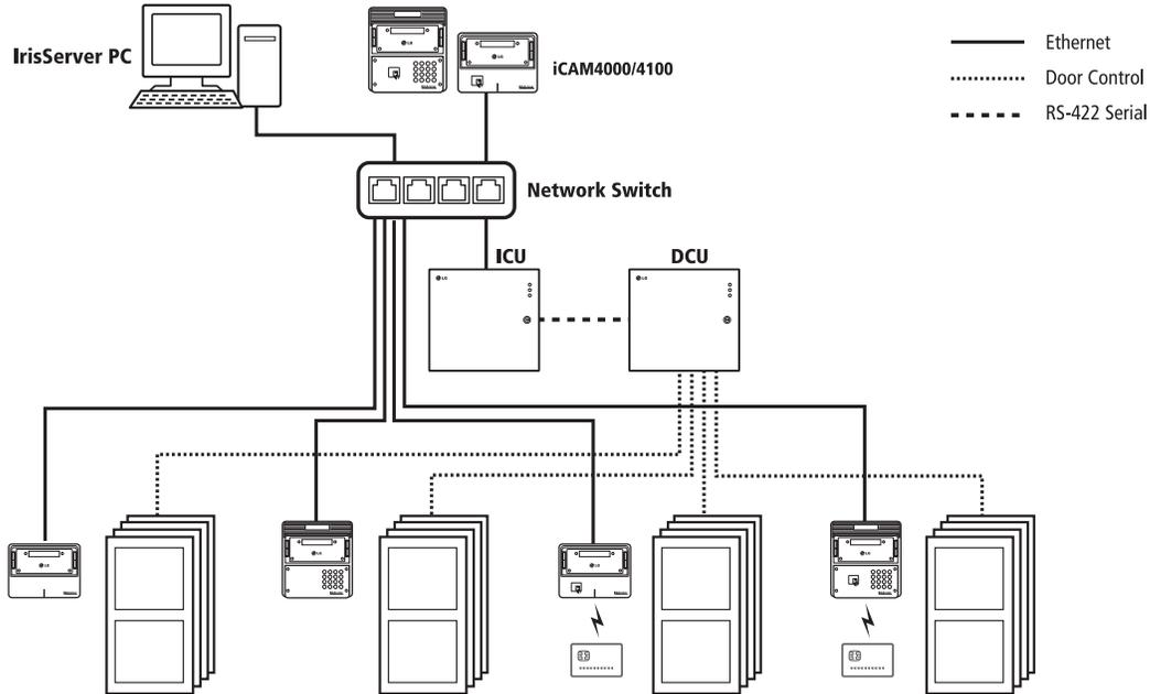
The iCAM4000 is a two-eye iris camera used to capture the iris images of the user. The iCAM includes an alignment indicator behind the mirror and voice prompts to assist the user. When used in a typical access control application, the iCAM will be placed near the secured portal and provides the means for the system to identify the user requesting entry.
