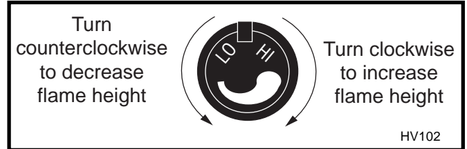
Fig. 38 Flame adjustment knob for Honeywell valve.
