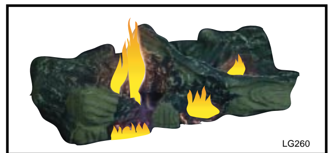
Fig. 40 Correct flame appearance.
