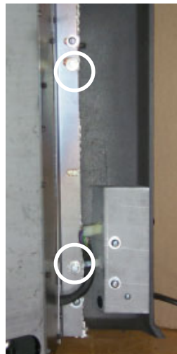
Rear View: Side panel attached with 2 bolts.
