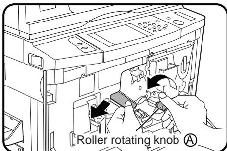
② Turn roller rotating knob **A** in the direction of the arrow to remove the misfed paper.
