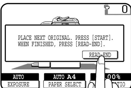
**9** After all originals are scanned, press the “READ-END” key on the touch panel.
