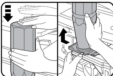
**7** Tap on the top of the toner cartridge 5 times to start the flow of toner into the toner hopper.
