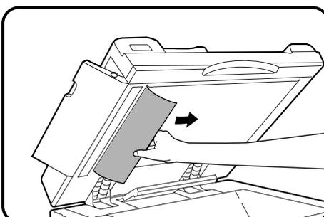
(C) Open the feeding roller cover and the document feeder cover, and remove the original.
