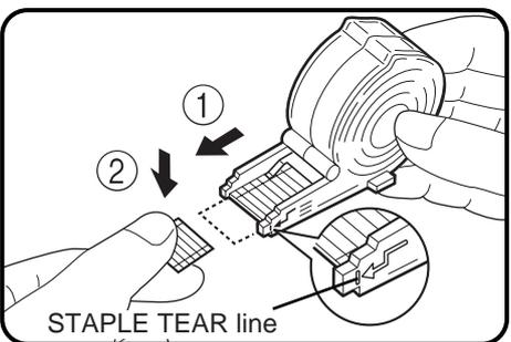
**4** Check that the first staple in the new cartridge is at the tip of the cartridge.
