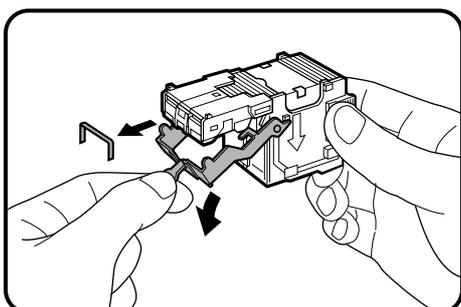
**5** Lower the lever at the end of the staple box and remove the jammed staples.
