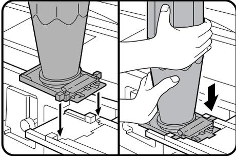
**4** Place the new toner cartridge with the tabs in the notches as shown.
