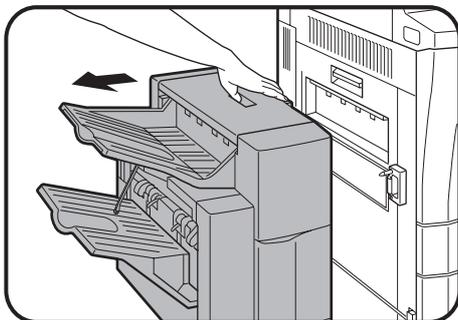
**2** While holding the finisher release lever, slide the finisher away from the copier.
