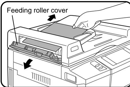
(A) Open the feeding roller cover and pull the original gently to the right and out from the document feeder tray.
