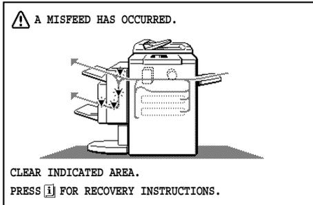
The copier will stop when a misfeed occurs. The message "A MISFEED HAS OCCURRED. CLEAR INDICATED AREA. PRESS **i** FOR RECOVERY INSTRUCTIONS." will appear along with a display of paper misfeed locations. Press the INFORMATION (**i**) key for more detailed information.
