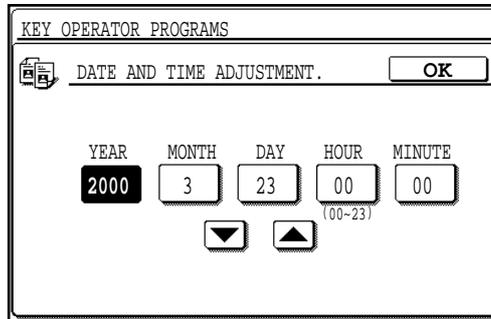
1. Select an item to be adjusted and adjust the value using the ▼ and ▲ keys.
