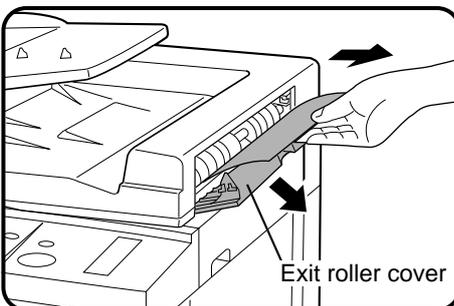
(B) Open the exit roller cover and gently pull the original out.
