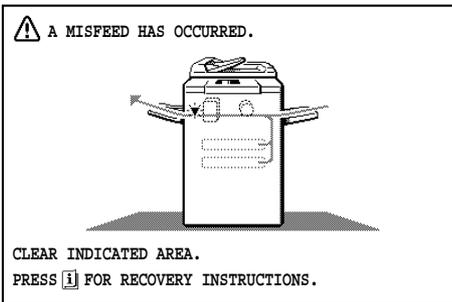
Misfeed around the fusing unit and exit area
