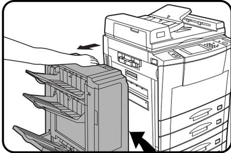
**1** While holding the finisher release lever, slide the finisher away from the copier.
