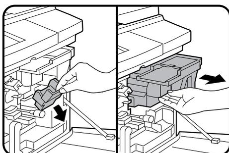
**2** Pull down the toner hopper lock lever and pull the toner hopper out slowly until it stops.
