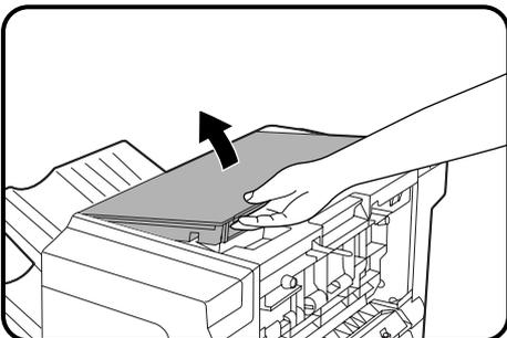
**5** If the misfed paper cannot be removed in step 4, close the cover of the paper feed area and open the top cover.
