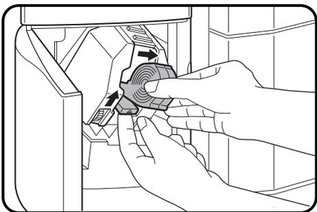
**2** Lift the green release lever and remove the staple cartridge from the stapler.
