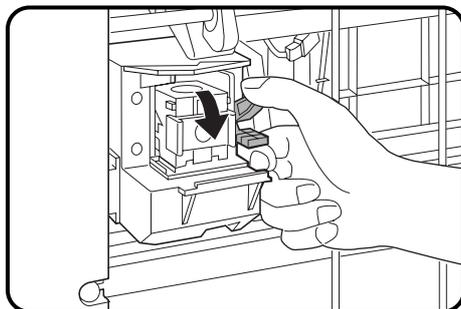
**3** Hold the staple box release lever to unlatch the staple box.
