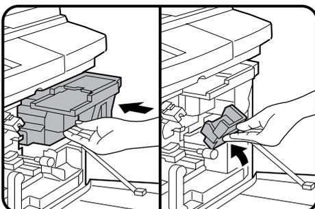
**9** Slide the toner hopper into the copier and return the toner hopper lock lever into place.
