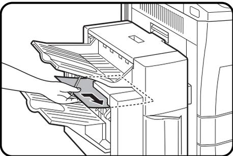
**3** Insert a new sheet of paper (A4 or 8-1/2” x 11” size) to the tray as shown in the picture to make the stapler work properly.
