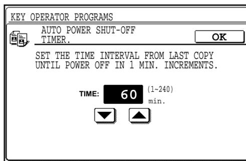
1. Enter the time interval using the ▼ and ▲ keys.
