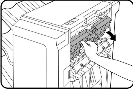
**3** If the misfed paper cannot be removed in step 2, open the cover of the paper feed area of the finisher.
