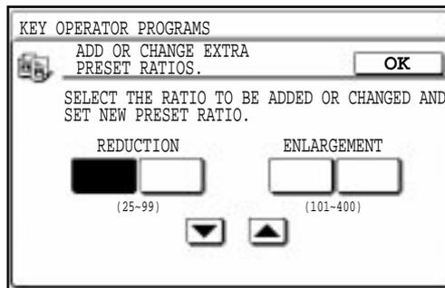
1. Press a key under "REDUCTION" or "ENLARGEMENT" on the touch panel.
