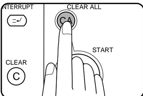
**8 To exit the key operator program mode, press the CLEAR ALL (CA) key.**
