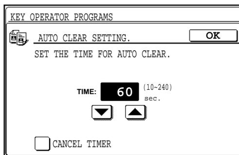
1. Set the desired time interval using the ▼ and ▲ keys.
