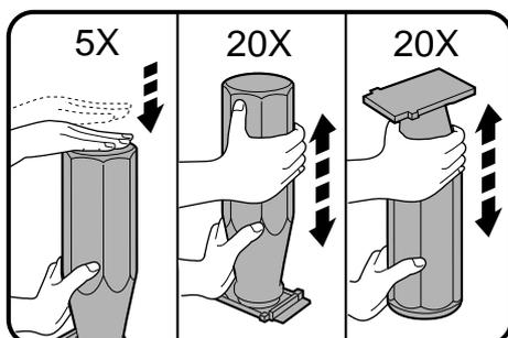
**3** Tap on the top of the toner cartridge 5 times. Hold the new toner cartridge vertically and vigorously shake it up and down about 20 times, then invert the cartridge and again shake it up and down about 20 times. This will loosen the toner and allow it to flow more easily into the toner hopper.
