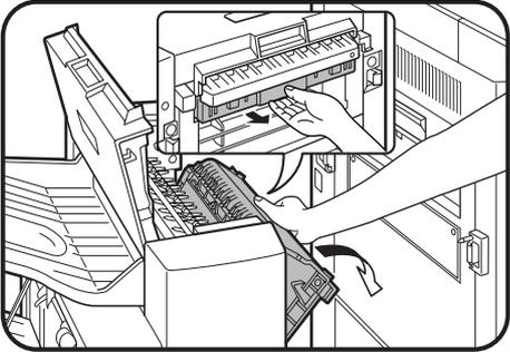
**6** Rotate the paper feed area cover as shown to open it.
