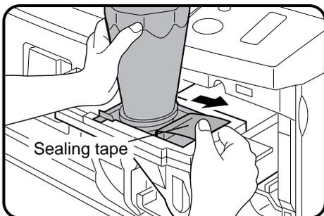
**6** Hold the toner cartridge with one hand while pulling on the sealing tape to remove it.
