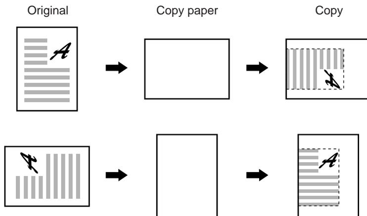
To enable rotation copy, press the check box of "ROTATION COPY SETTING." to display a check mark in the check box. To disable this mode, press the check box of this program again to clear the check mark in the check box.
