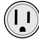
Two-Pole, 3-wire Grounding Receptacle 15 Amps. 125V.
