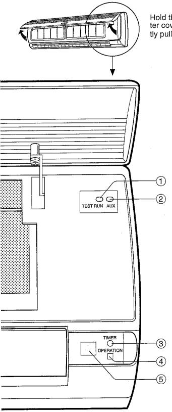
Hold the bottom corner of the filter cover on both sides and gently pull outwards.
