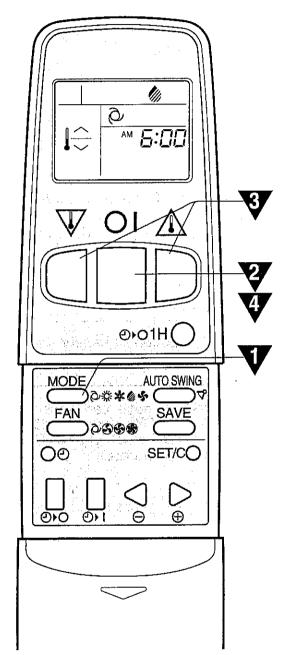
In the DRY mode, the air conditioner reduces the humidity in the room without lowering the room temperature.
