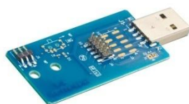
Figure 6: uSSD External USB Adapter
