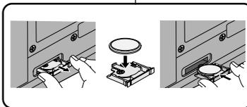
**Note:** The battery holder will only fit one way to avoid possible incorrect insertion.
