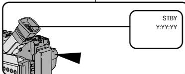
When a cassette is loaded and the camcorder is left in STANDBY mode for over 5 minutes without being used, it will turn off automatically. To use it again, push the red START/STOP button or set power switch to OFF and then back to CAMERA. This Auto Power Off feature is designed to save battery power and to protect the Tape Head and tapes.
