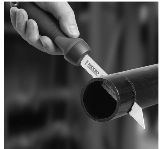
Jab Saw cutting through PVC
