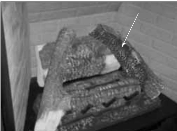
Figure 14.14 Positioning Right Log
