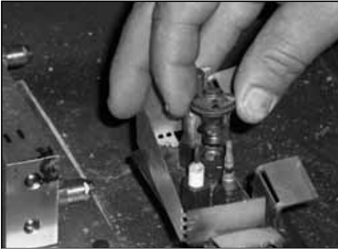
Figure 11.5 Remove Pilot Hood
