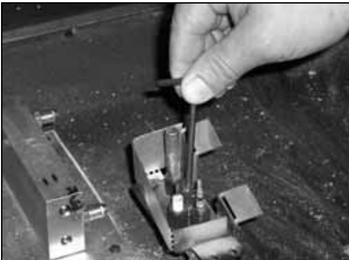
Figure 11.6 Remove Pilot Injector
