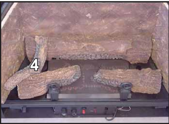
Log #4 (srv340-705): Rest log #4 in the left smooth cut-out area on the end of log #1 and place the lower end on log #2. The left end and “bump” of log #4 both rest on log #2.
