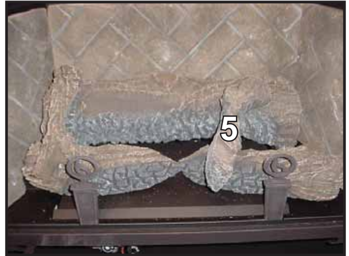
Log #5 (srv340-706): Place log #5 across log #1 and log #3. The notch in the bottom of the log sets on the carved out edge on top of log #3. The back of the log sits in the grooved out area in log #1.
