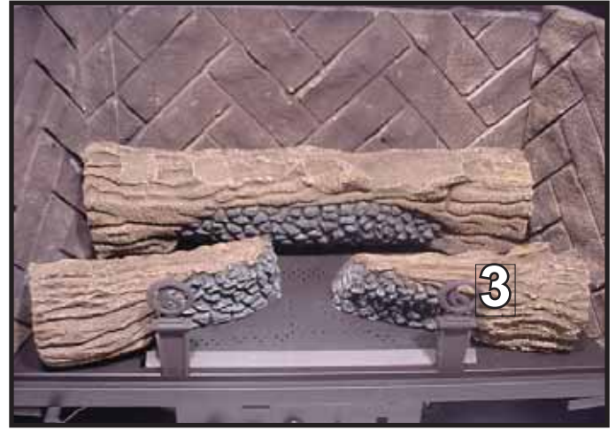
Log #3 (srv330-703): Position log #3 by locating its slot over the tab on the right front of the burner. The right end of log #3 is pushed up against the step in the base pan.
