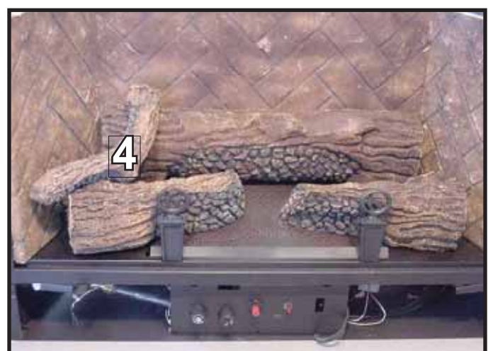
Log #4 (srv340-705): Rest log #4 in the left smooth cut-out area on the end of log #1 and place the lower end on log #2. The left end and “bump” of log #4 both rest on log #2.
