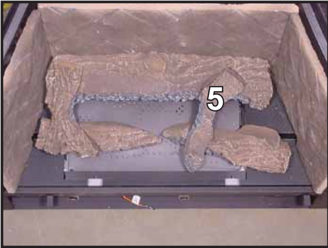
Log #5 (srv340-706): Place log #5 across log #1 and log #3. The notch in the bottom of the log sets on the carved out edge on top of log #3. The back of the log sits in the grooved out area in log #1.
