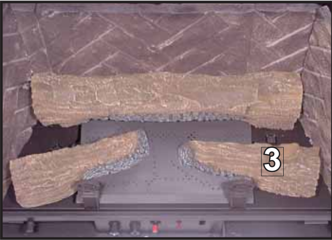
Log #3 (srv330-703): Position log #3 by locating its slot over the tab on the right front of the burner. The right end of log #3 is pushed up against the step in the base pan.
