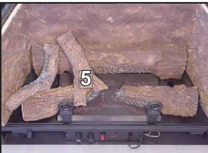
Log #5 (srv330-704): Rest log #5 in the second smooth cut-out area on the end of log #1 and place the lower end on log #2. The “Y” end of the log sits on the right end of log #2.
