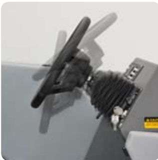
The tilt steering wheel is just one of the features that provide operator comfort and ensures optimal vision
