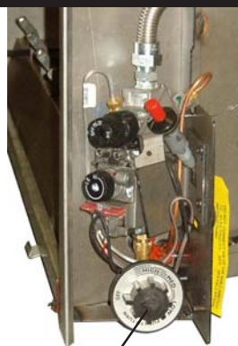
rear burner control knob
