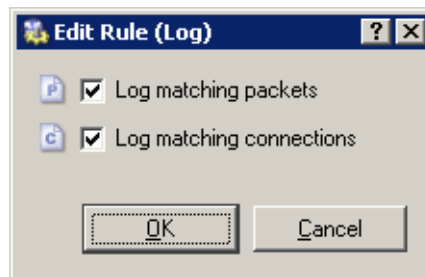
Figure 6.18 Traffic rule — packet/connection logging
