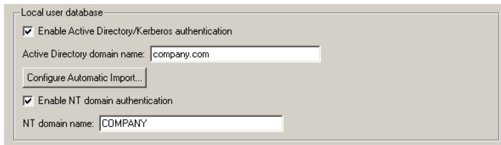
Figure 23.3 Setting of NT authentication for local user accounts
