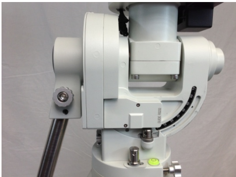
Figure 17. Tilt the counterweight shaft for low altitude
