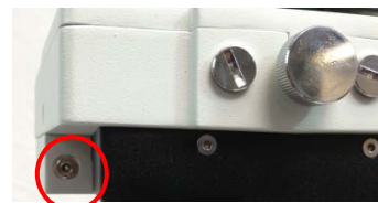
Figure 3. LED reticle on DEC unit
