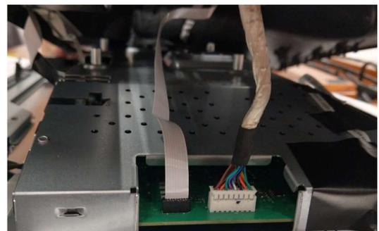
**S9** Tear off a tape from CTRL FFC cable on Rear Cover
