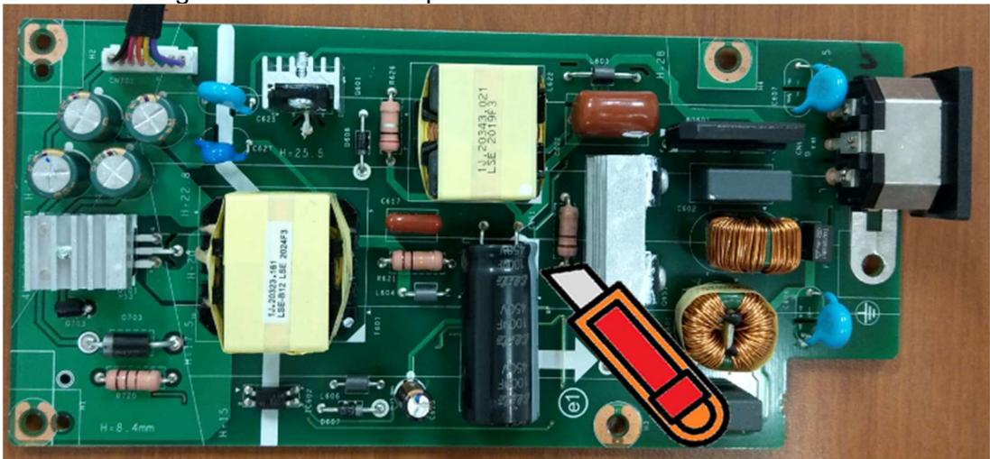
S38-2 Ensure cutting path within the glue, don't touch bulk cap. or PCB
