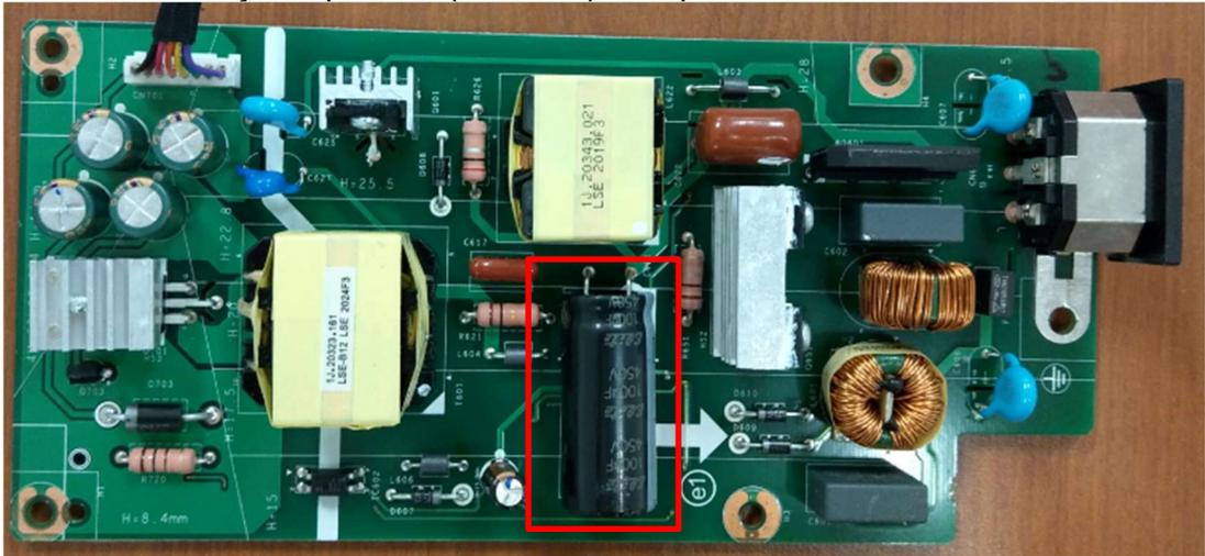
S38-1 Cut the glue between bulk cap. and PCB with a knife
