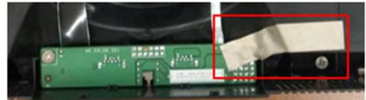
**S16** Unlock 2 screws to disassemble USB BD from Rear Cover
