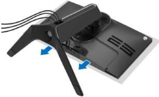
**S3** Disconnect the cables from the monitor and slide them out through the cable-management slot on the stand riser
