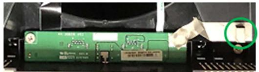
**S15** Remove a conductive cloth from the right USB screw and Rear Cover
