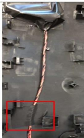
**S14** Remove a conductive foam from conductive cloth
