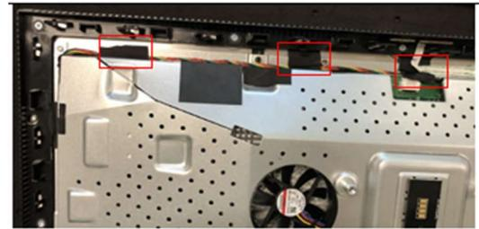
**S18** Remove FFC cable from Rear Cover, CTRL BD and CTRL+KEY BD
