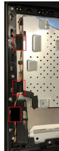
**S20** Disconnect "CTRL+LENS BD FFC" from I/F BD and remove it from Panel and Main SHD
