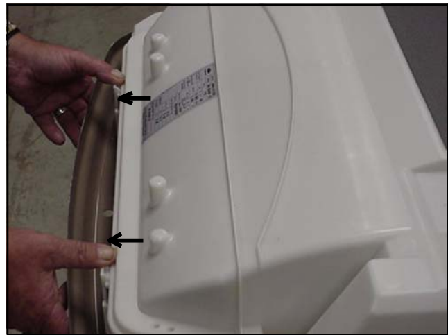
Figure 3-29 Upper Scroll Assembly Keeper Tab Release
