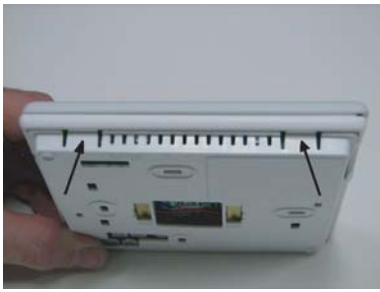
Fig. 4 - Press Tabs to Remove Backplate
