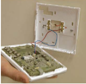
Fig. 9 - Connect Pigtail Wires to Display Module
